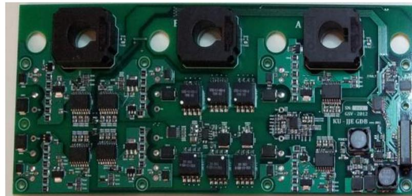
**110kW PowerPC based DC/AC Inverter for EV**
