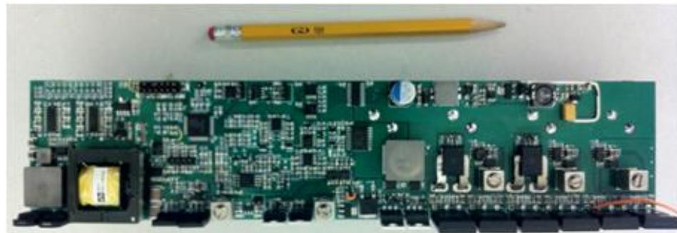
**48V/4kW Inverter + 100W E Alternator**
